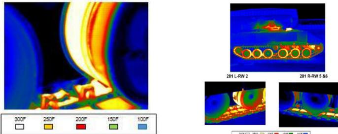
The dramatic increase in temperatures is attributed to the hysteretic properties of the tank track elastomers.
